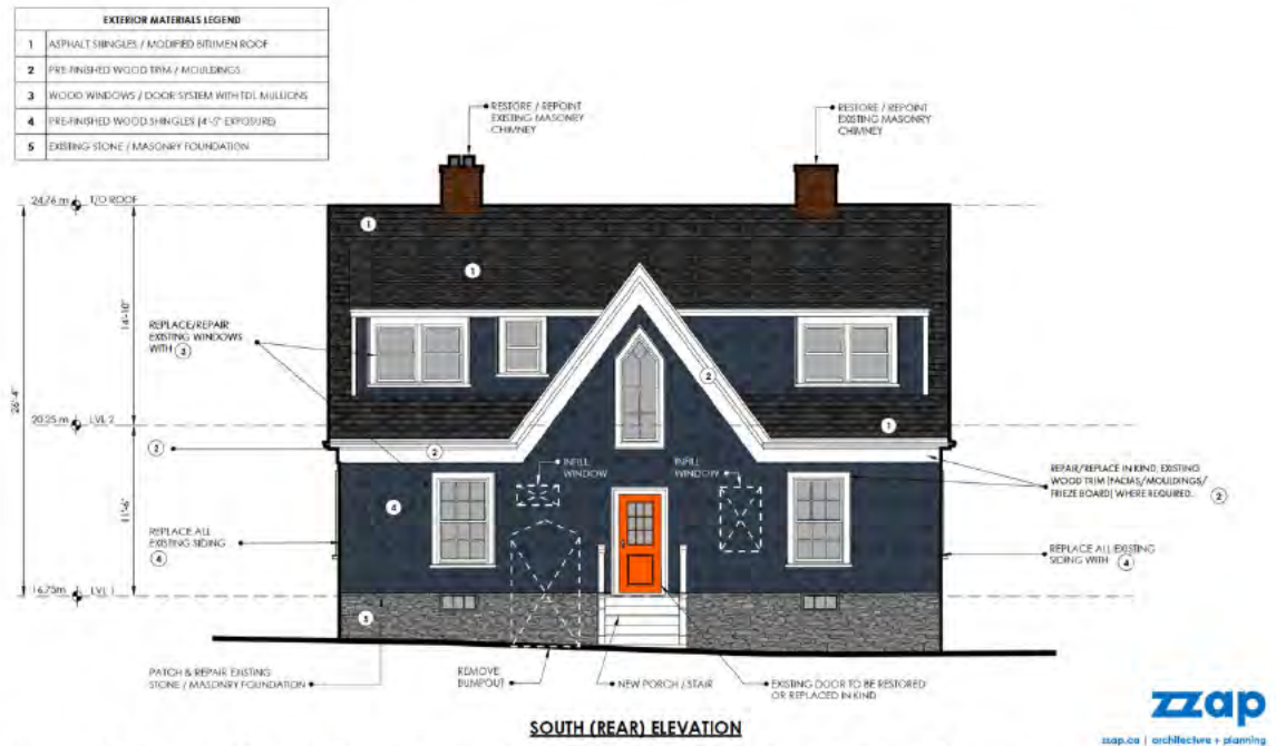
Figure 45: South (Rear) Elevation – George and Mary Shiels Residence (Restored)
