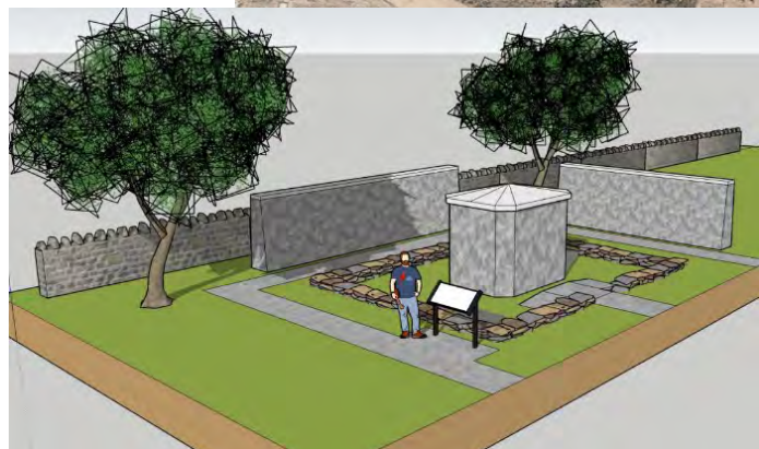
Figure 2: A 3D model providing a conceptual example of how the 1846 stone foundations and the northern stone masonry wall can be sensitively incorporated into the design of a new columbarium. Note: Conceptual only; not a final design proposal.
